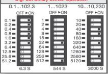
The TDU is an encapsulated solid state delay on make timer that combines digital timing circuitry with universal voltage operation. It offers DIP switch adjustment allowing accurate selection of the time delay over the full time delay range. Encapsulation protects against humidity, vibration, and dust making it suitable for outdoor equipment installations. This series is an excellent choice for OEM equipment where fast, positive adjustment, low cost and long life are important.
