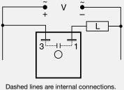
Load may be connected to terminal 3 or 1.
