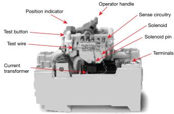
ABB Residual Current Device
