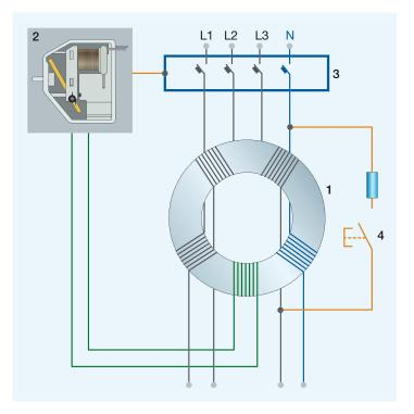
The energy required by internal relay to open ABB GFEP contacts is only 25µVA (approximately 1/40.000 W).
